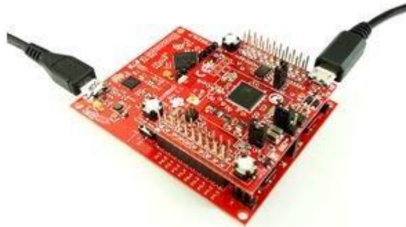
Fig17: CC3100 mounted on MSP430
